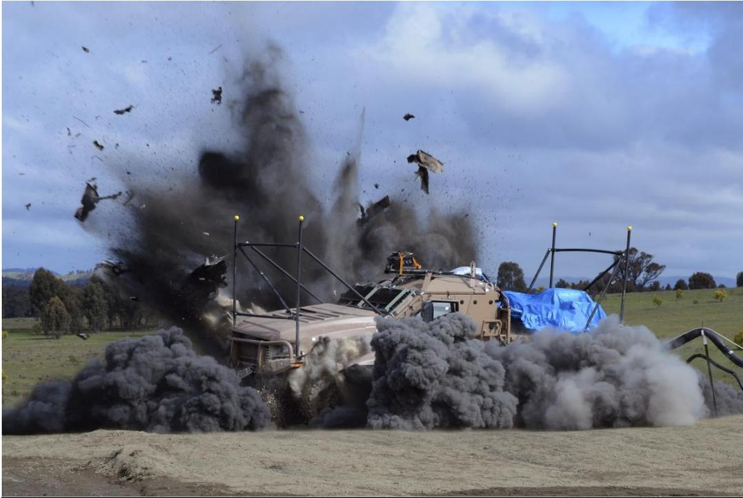
A Hawkei is subjected to a live-fire underbelly blast testing during trials in 2011
