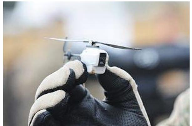
The UAV is equipped with a camera, which gives the operator full-motion video and still images.
