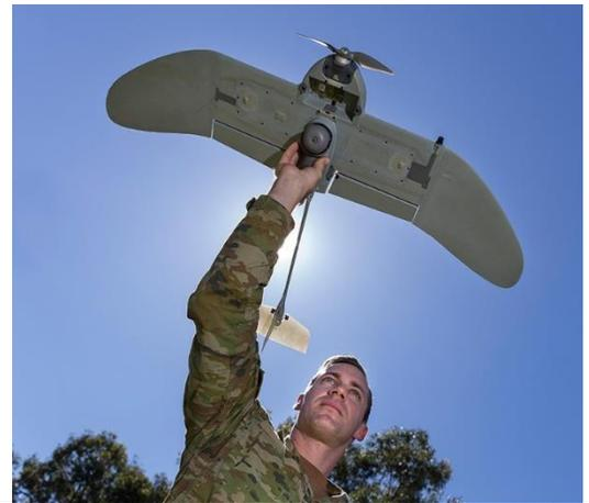
The Wasp AE weighs 2.8 pounds, operates for up to 50 minutes at a range of up to five kilometers and delivers live, streaming color and infrared video from its pan-tilt-zoom Mantis i22 AE gimbaled payload. Launched by hand and capable of landing on the ground or in fresh or salt water, the Wasp AE provides portability and flexibility for infantry, littoral or maritime reconnaissance operations. Photo: Sgt. Janine Fabre, Australian Defence
